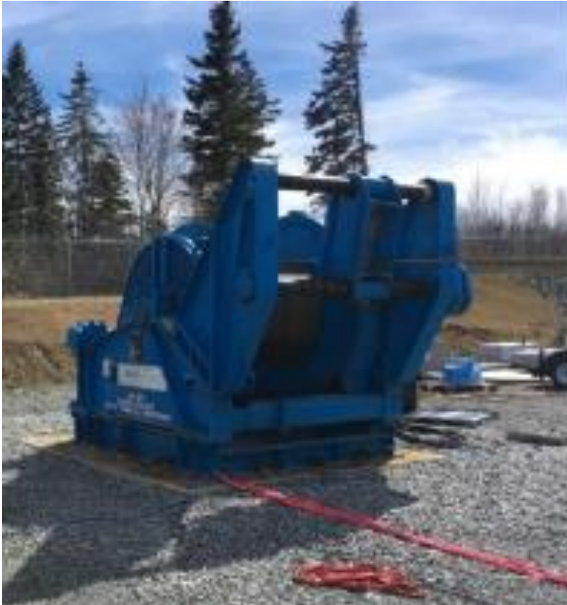
Figure 6.12: Photograph of typical onshore cable pull-in winch
